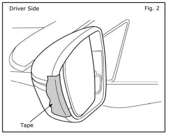
Apply protective tape to outer edge of mirror housing as shown to protect it from damage while removing mirror glass assembly.
