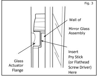
Looking in through edge of mirror housing, locate intersection between flange of glass actuator and back wall of mirror glass Assembly. Insert a pry stick with a narrow tip or a flathead screwdriver and carefully pry off glass assembly.
