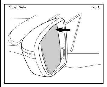
1) Adjust driver side mirror so glass is tipped inboard as much as possible. This will expose access point for removing existing glass assembly from mirror housing.
