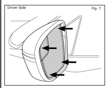
7) Using even pressure, press firmly on new glass assembly to seat it into mirror housing. Take care that initial force applied is **perpendicular** to Mirror Housing. You will hear and feel a definitive snap as mirror glass assembly engages with glass actuator.
